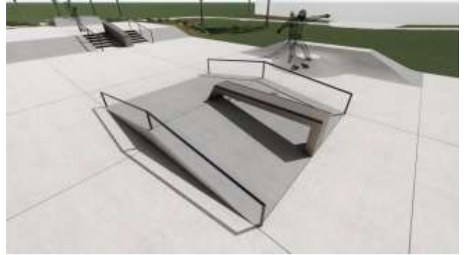
Bank to bank with low/ high A frame rails and central ledge [10]
