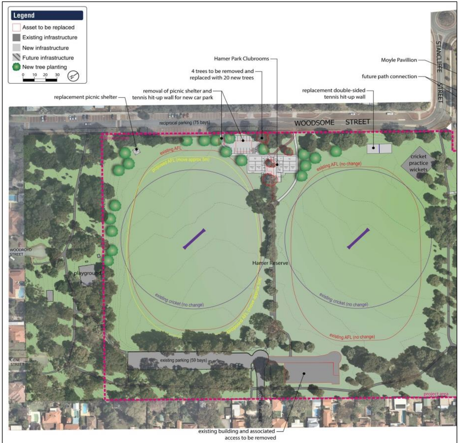
Figure 1: Hamer Park Section - Building Site Plan
