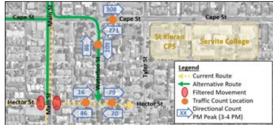
Figure 2(b). Alternative Access Routes and Existing Directional Traffic Counts in PM Peak 3pm-4pm
