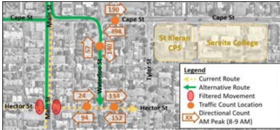
Figure 2(a). Alternative Access Routes and Existing Directional Traffic Counts in AM Peak 8am-9am
