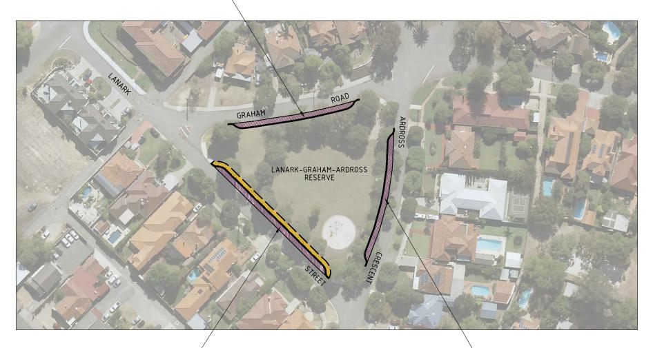
60.9m PARALLEL PARKING EMBAYMENT, SUFFICIENT FOR APPROXIMATELY 12 CARS REMOVAL OF 6 MATURE TREES - 60.9m PARALLEL PARKING EMBAYMENT, SUFFICIENT FOR APPROXIMATELY 10 CARS REMOVAL OF 6 MATURE TREES
