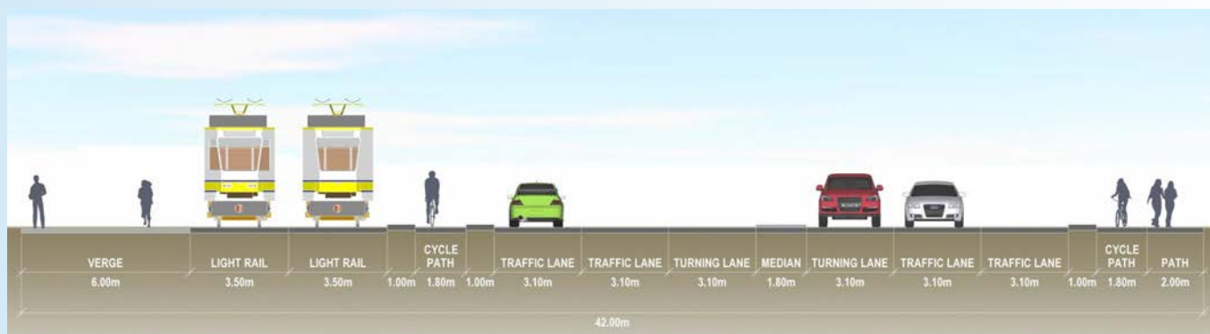
Figure 30: Stephenson Avenue Cross Section – Stephenson Bridge
