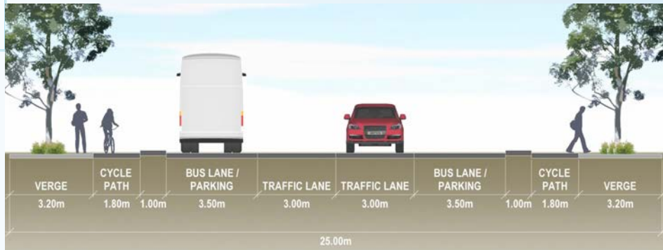
Figure 39: Howe Street Cross Section (between King Edward Road and Stephenson Avenue)
