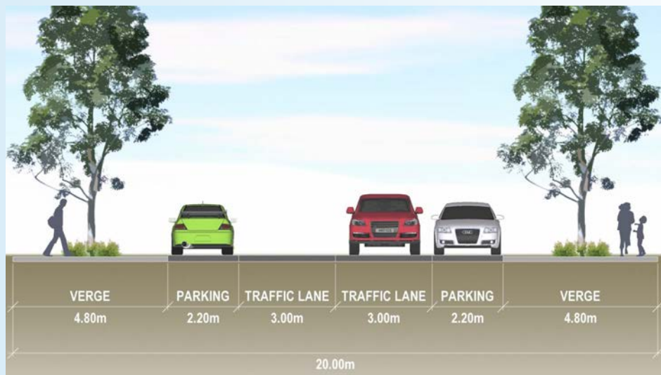
Figure 37: Oswald Street Cross Section (East of Stephenson Avenue)
