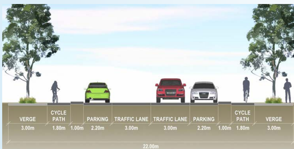
Figure 38: Oswald Street Cross Section (West of Stephenson Avenue)
