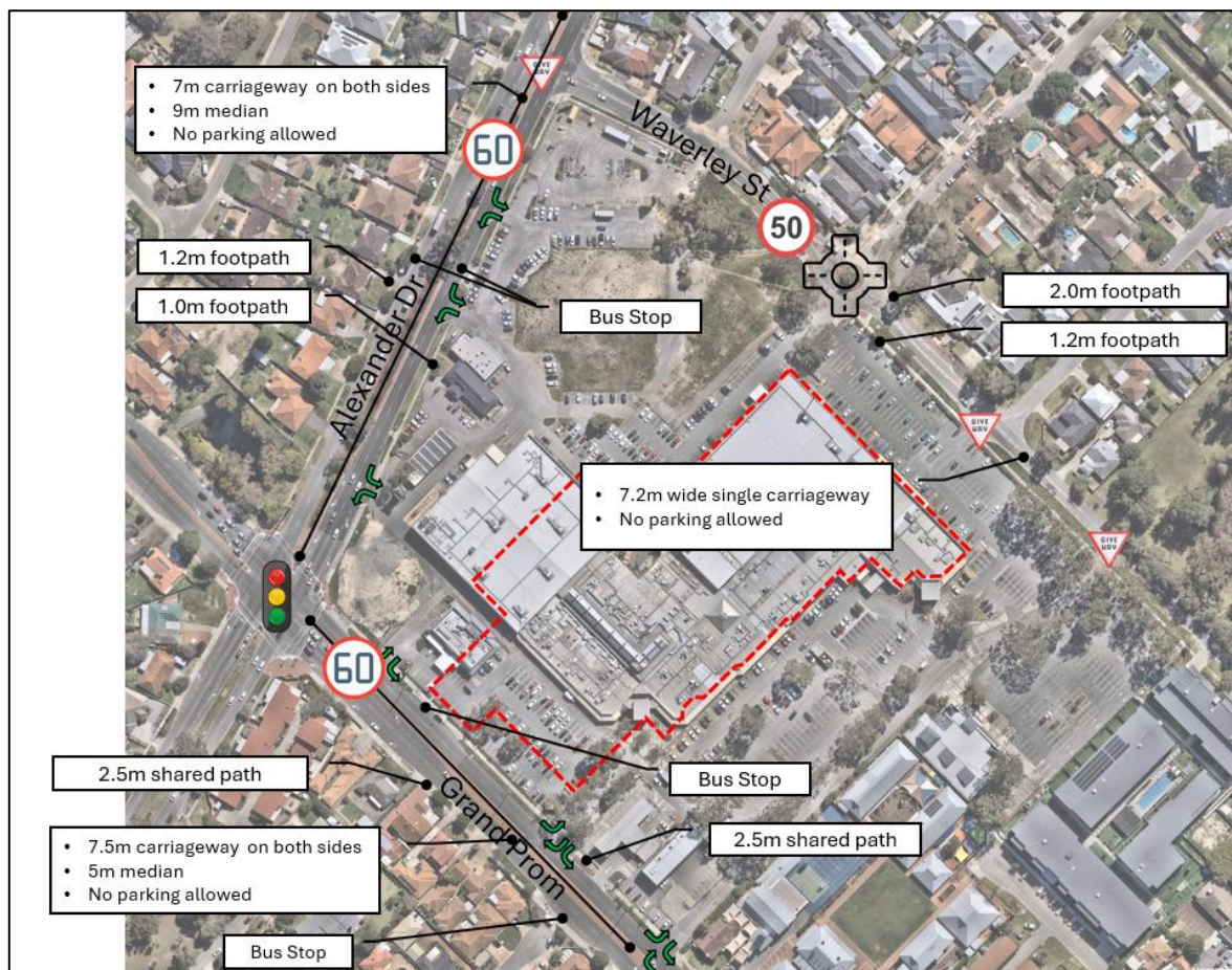
Figure 2-6: Current Traffic Management Fronting Site
