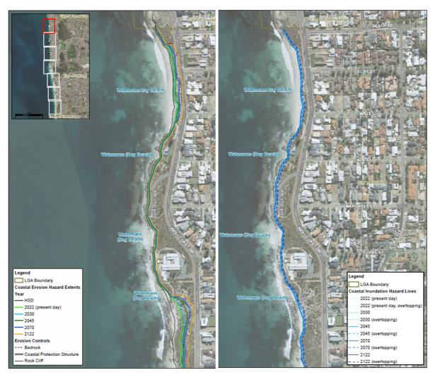
Figure 3.3 MU1 – Coastal Erosion & Inundation Hazards
