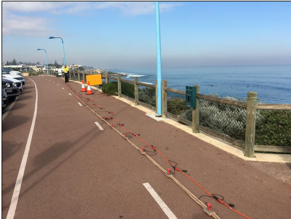
Figure 2: MASW data acquisition along the shared path on the western verge of West Coast Drive.
