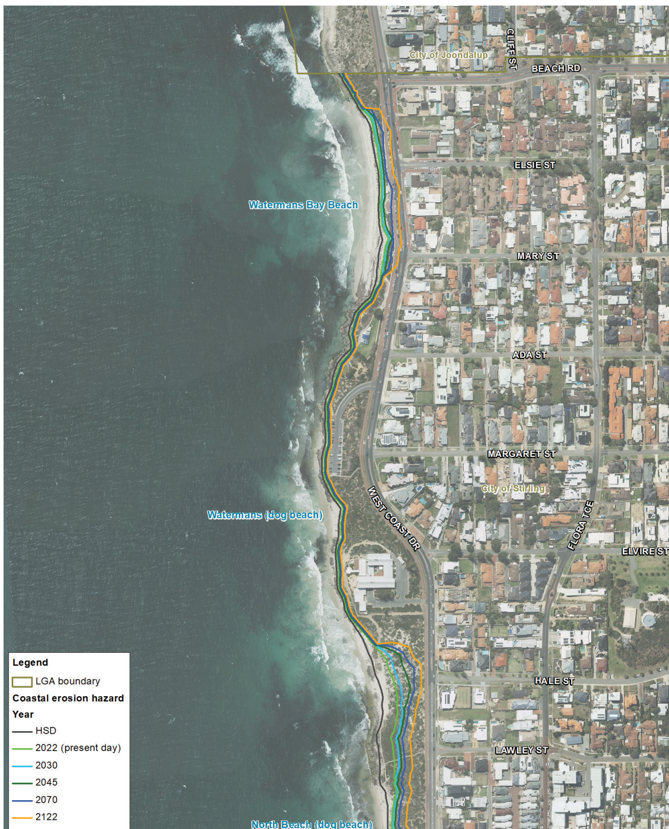
Figure 4a: Coastal erosion lines zone 1
