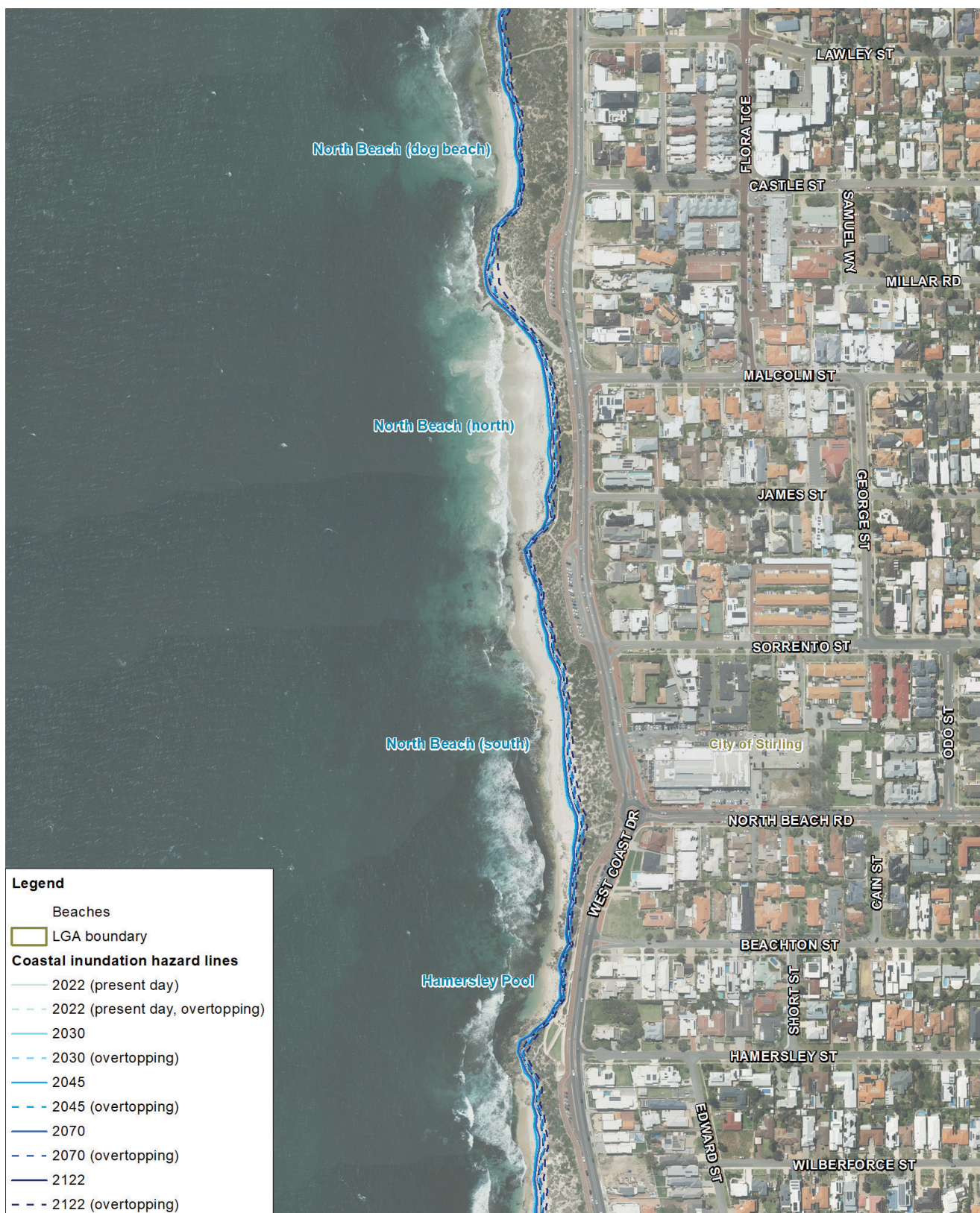
Figure 4k: Coastal inundation lines zone 2
