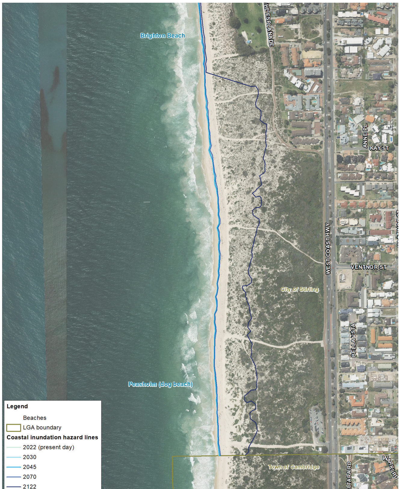
Figure 4p: Coastal inundation lines zone 7
