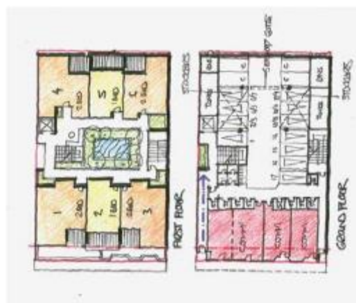
Ground and first floor plans, showing parking, offices and courtyard apartments.
