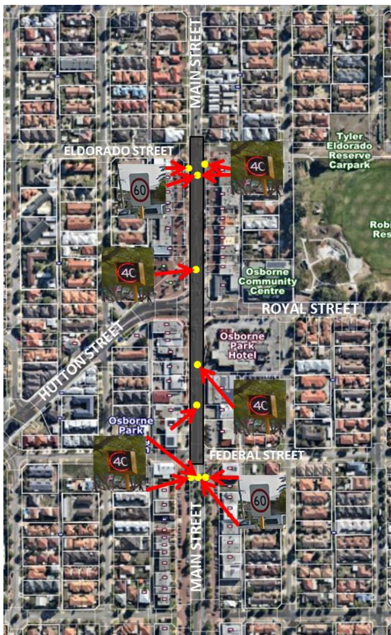
Figure 4 – Current locations of 40km/h variable speed signs and 60km/h signs in the Main Street Town Centre
