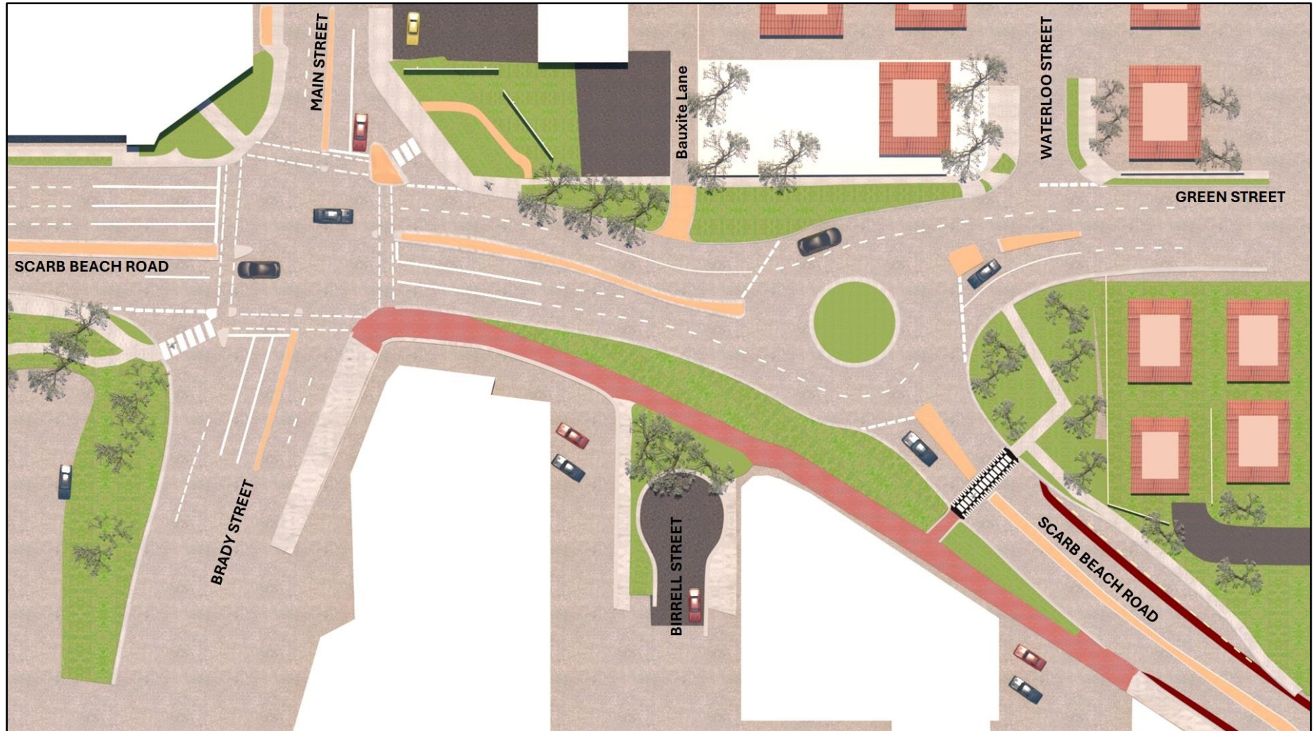
Figure 1 - Concept Design Plan of Proposed Intersection Modifications
