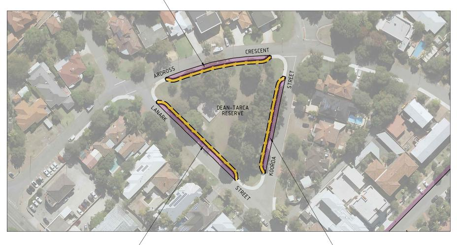
68.6m PARALLEL PARKING EMBAYMENT, SUFFICIENT FOR APPROXIMATELY 11 CARS REMOVAL OF 5 MATURE TREES - 60.5m PARALLEL PARKING EMBAYMENT, SUFFICIENT FOR APPROXIMATELY 10 CARS REMOVAL OF 2 SIGNIFICANT MATURE TREES
