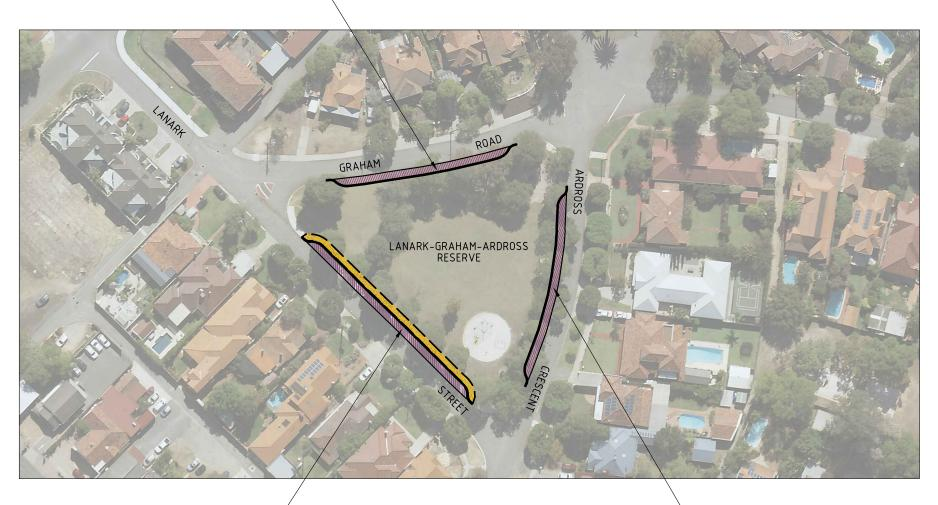
60.9m PARALLEL PARKING EMBAYMENT, SUFFICIENT FOR APPROXIMATELY 12 CARS REMOVAL OF 6 MATURE TREES - 60.9m PARALLEL PARKING EMBAYMENT, SUFFICIENT FOR APPROXIMATELY 10 CARS REMOVAL OF 6 MATURE TREES
