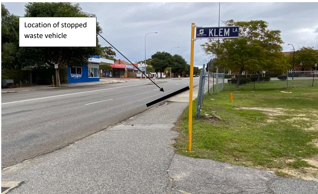
Finding 2.4 – Sight lines from Klem Lane looking northwest along Walcott Street – potential for stopped waste vehicle to restrict sight lines
