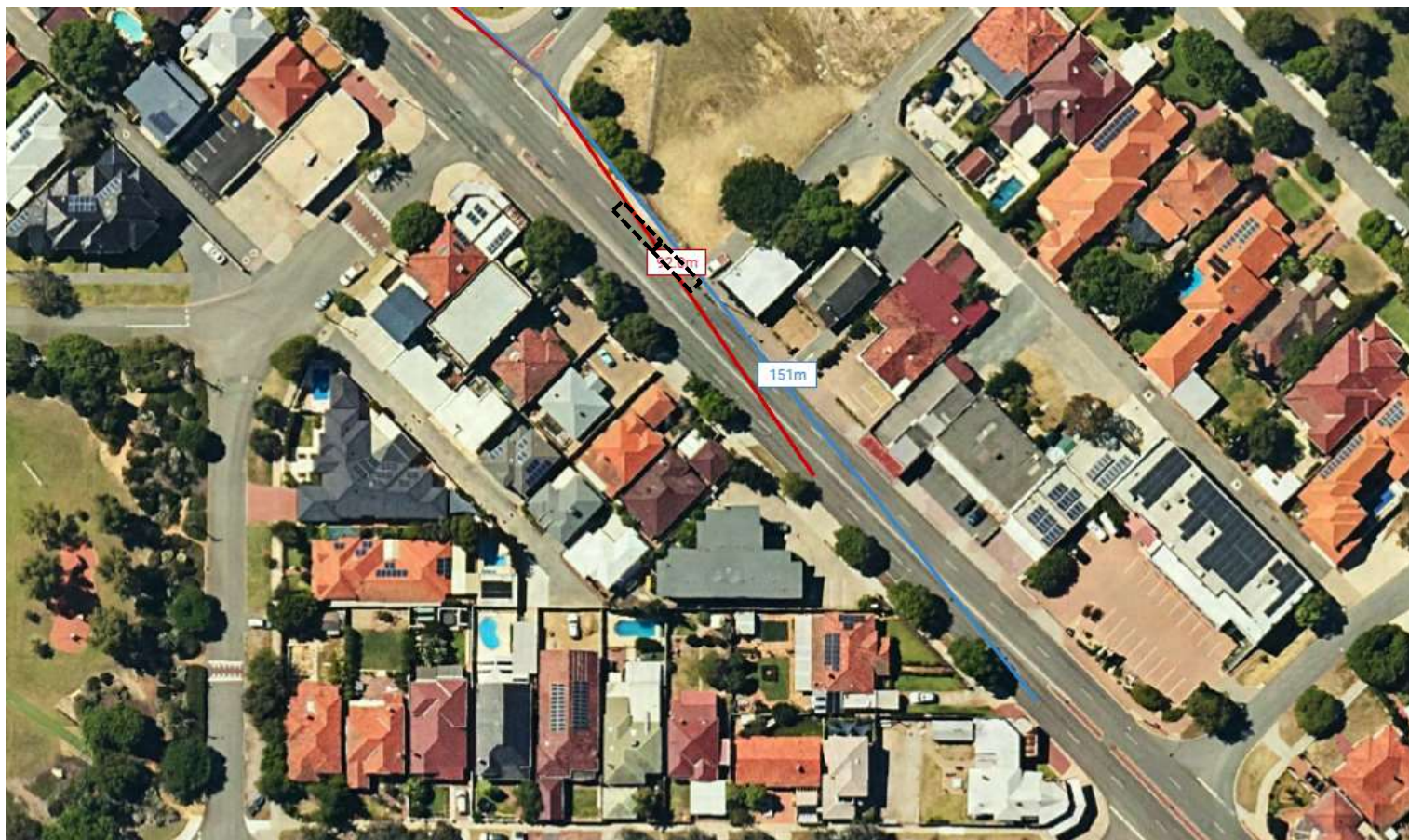
Finding 2.4 – SISD (blue) and SSD (red) from Adair Parade looking southeast along Walcott Street – potential for stopped waste vehicle to restrict sight lines. Finding 2.9 – potential for on street parking to also restrict sight lines
